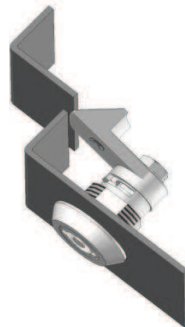
cam will move upright when touches the body
